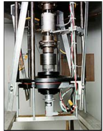
Motor test train mounted on lid of spin test tank located in the Power Electronics Laboratory.
